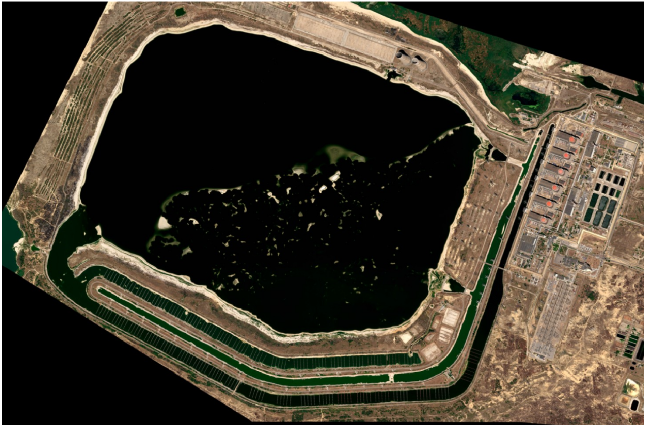
Satellite image of the Zaporizhzhia nuclear plant showing the six reactor units and cooling pond and water inlet and outlet channels, and electrical switchyard (right side of image) 12 August 2025. Source: © Airbus DS 2025
